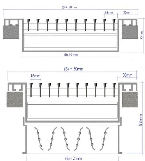
The supply linear bar grille is a wall mounted supply grille used in cooling, heating or air ventilation applications.
