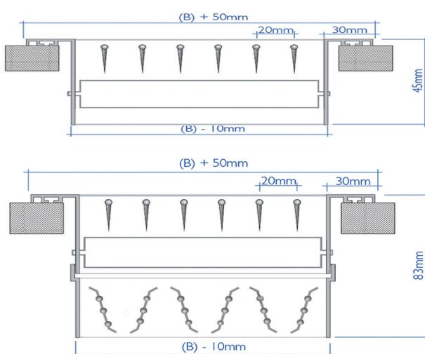
Double Deflection Grille is a type of grilles with a two set of blades - vertical and horizontal - used to deflect air in both the horizontal and vertical directions. DDG is a grille without opposed blades damper (OBD) and is commonly used as a side wall return air grille. DDR is provided with opposed blades damper (OBD) to facilitate precise air volume control. DDR is usually used as a supply air register on side wall applications.
